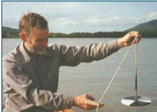
A volunteer lay monitor uses a secchi disk to measure the water clarity of Lake Champlain.
