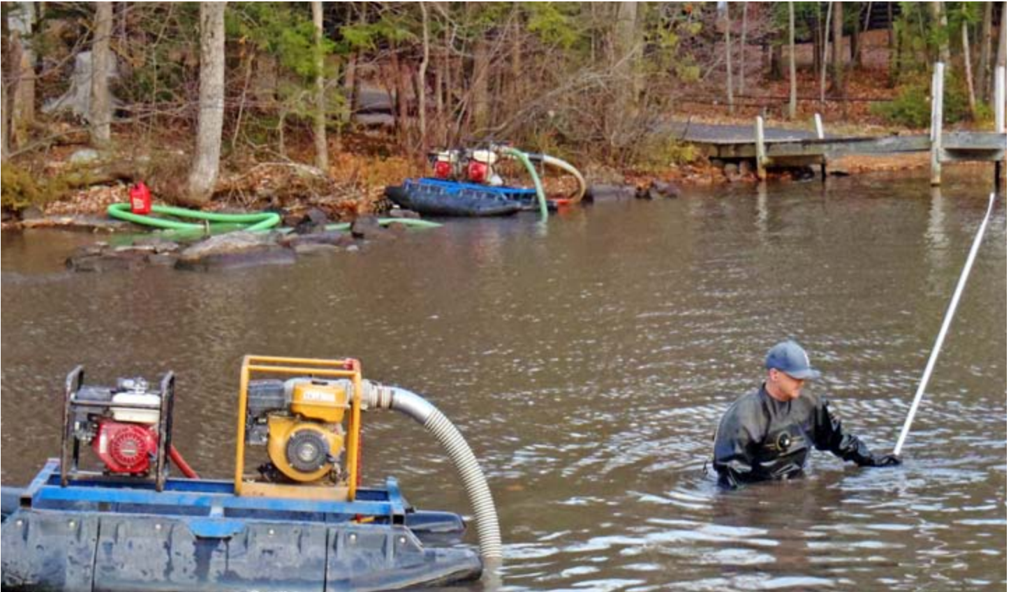
AquaCleaner staff suction harvesting at Middleworth Bay. Photo courtesy of Lake George Association
