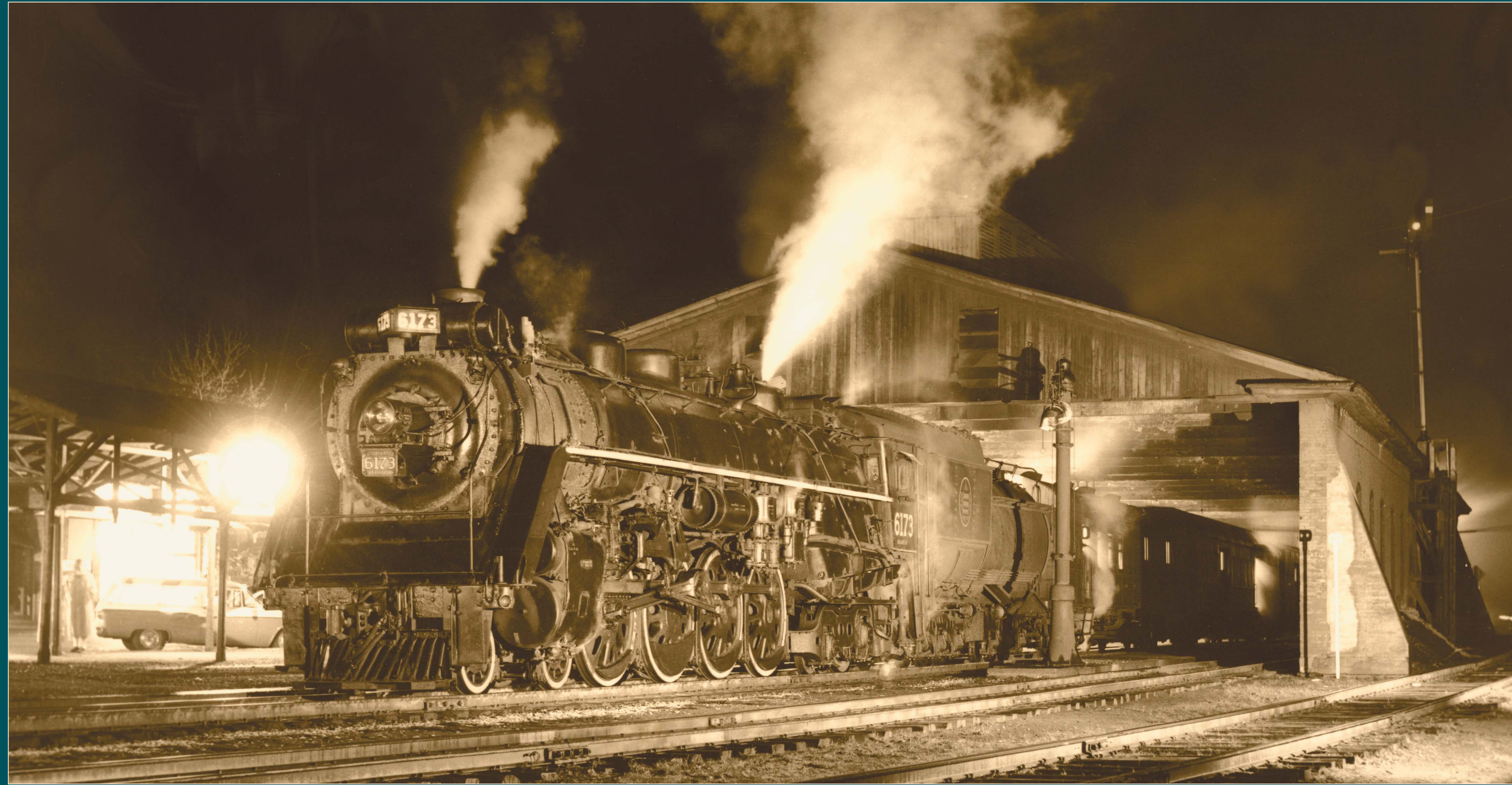
This photo, taken in 1956, shows Canadian National Railway steam locomotive #6173 which weighed over 400,000 pounds and put out about 3,000 Horsepower. Diesel engines, the standard today, were first introduced in 1941. The last steam engines ran through Essex Junction in 1957. The train shed was built in 1867 and stood for nearly 100 years.
