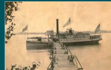
Built in 1882 and powered by an 800-horsepower steam engine, this 168 ft (51.2m) vessel ran between Burlington and Alburgh, VT. It sank in 1902, was salvaged to Whitehall, NY, cut for scrap and its hull sunk in nearby South Bay. Its turret house is on display at the Lake Champlain Maritime Museum in Ferrisburgh, VT.
