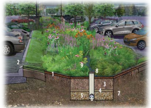
Parking lot 'bioretention' or rain garden to help absorb and treat stormwater.
