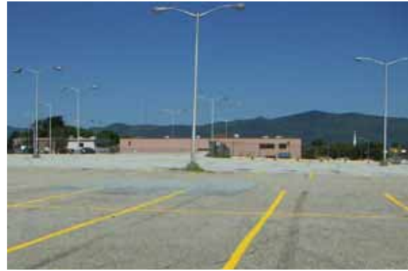
Rutland, VT. Stream health tends to decline with increasing impervious land cover; particularly when total imperviousness reaches a critical threshold. That threshold varies from stream to stream, but averages approximately 10% of a stream's drainage area.
