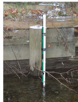
Figure 3. Typical FMP pressure transducer installation. The transducer is in the bottom of the PVC tube that is secured to the fence post.
