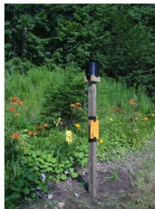
Figure 2. Typical FMP tipping bucket rain gage setup.
