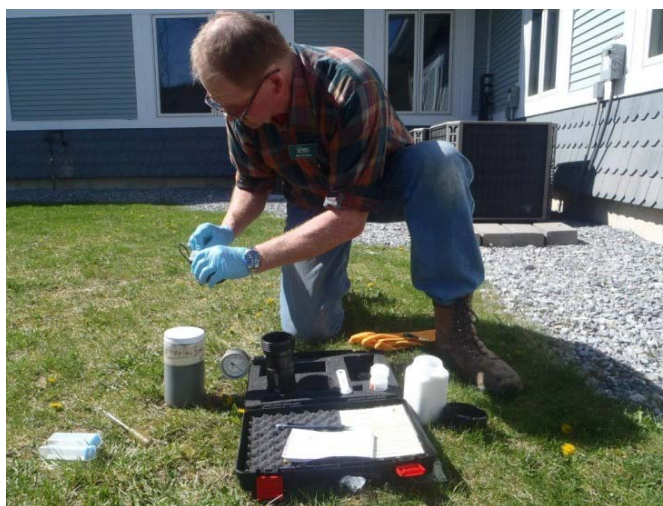
Agros manure test to determine N content.
