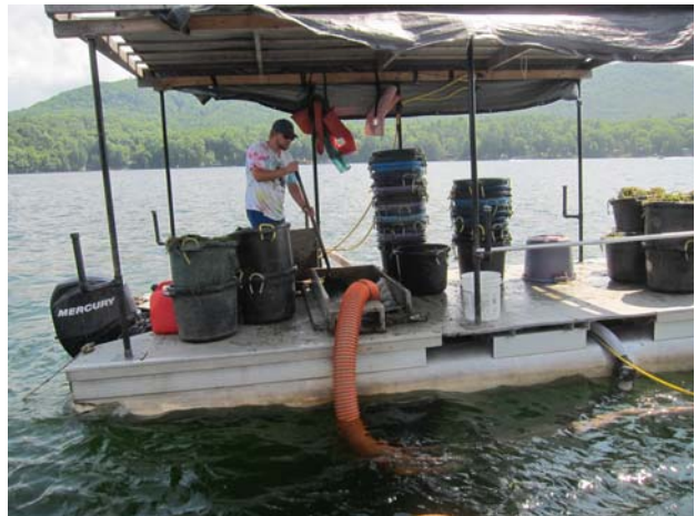
Eurasian water milfoil population control is a focus of the Lake Dunmore program. Here milfoil is removed with a suction harvester.
