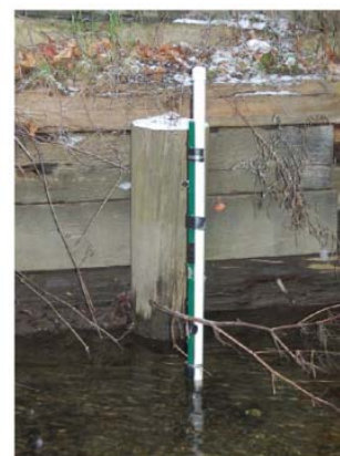
Figure 3. Typical FMP pressure transducer installation. The transducer is in the bottom of the PVC tube that is secured to the fence post.
