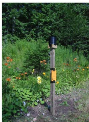
Figure 2. Typical FMP tipping bucket rain gage setup.
