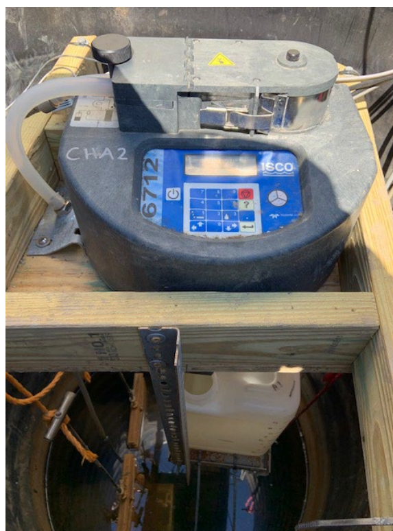
Figure 15. Custom autosampler rack in monitoring manhole
