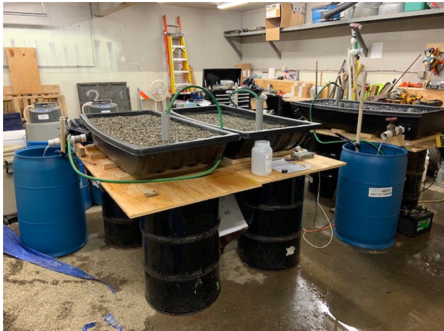
Figure 10. Three filter sleds recirculating P solution
