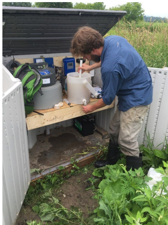
Figure 9. Processing a composite water sample
