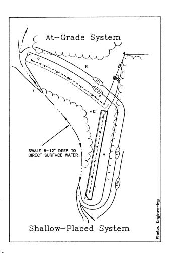
the site conditions, the separation distance of the disposal fields to the seasonal high ground water table was reduced from 24" to 18". The two units were angled slightly to fit the contour of the site. A valve at the effluent application point allows the effluent to be directed to one disposal system or the other.
