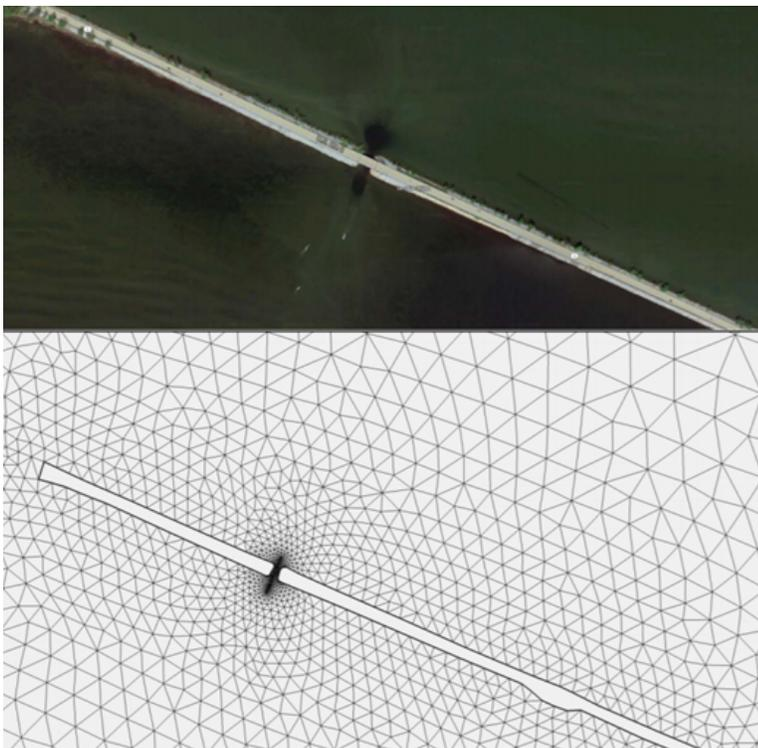
**Image:** Aerial photo of US highway 2 between South Hero and Colchester, Vermont, and the corresponding mesh used in the Lake Champlain-Richelieu River 2D Hydrodynamic Model to simulate the hydraulic effects of this structure on water levels in Lake Champlain.
