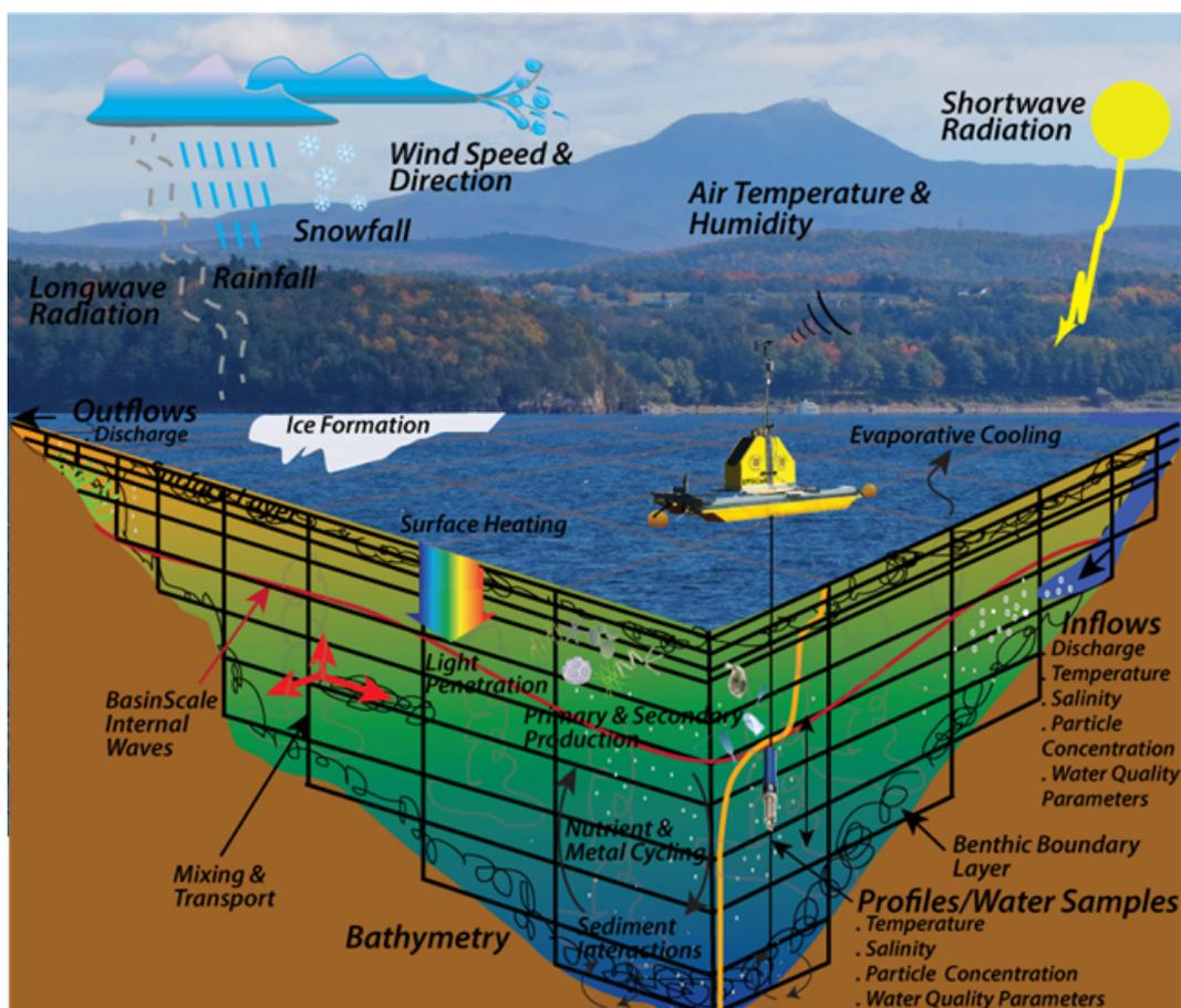
**Image:** Input data and key physical and biogeochemical processes simulated by the 3-D Coupled Hydrodynamic-Biogeochemical Model of Lake Champlain (Credit: Schematic developed by C. Marti)
