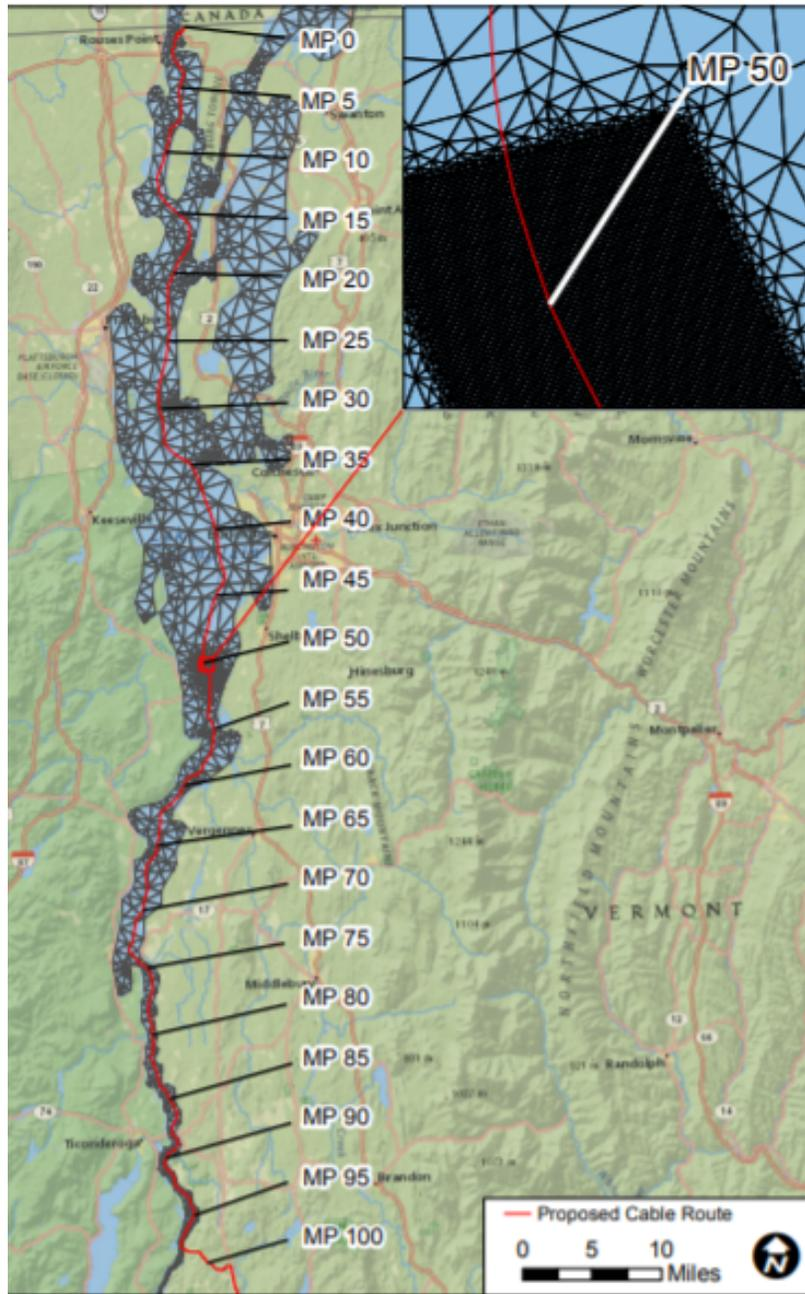
**Image:** Map shown in the Lake Champlain Water Quality monitoring report. Black lines over the lake demonstrate the model grid. The "MP" annotations refer to the mile point of the proposed cable length.
