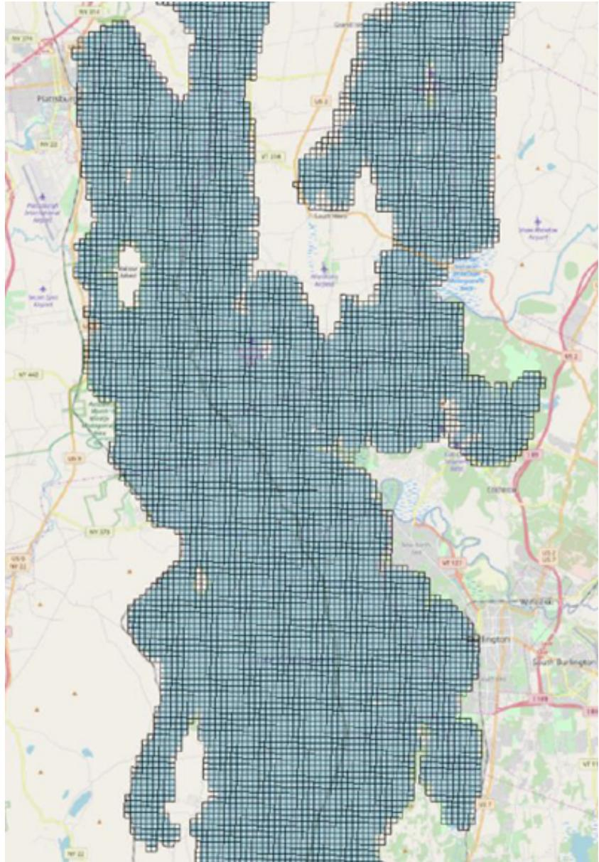
**Image:** Map view of Lake Champlain overlaid with the cells of the Deltares DFLOW-Flexible Mesh Hydrodynamic Model
