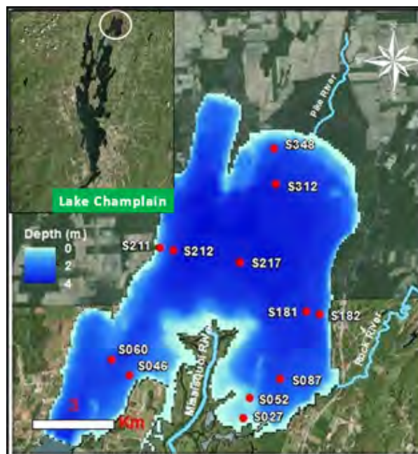
Figure 1. MB site and bathymetry map with sample core locations (red dots) where sectioned cores (to 10 cm) have been analyzed for P inventories at 4 time points in 2013 (June–Sept.). At point S087, there are biweekly time series of sediment P inventories in 2013-14 and 2014-2015. All points have coincident water column physical, chemical and biological data (Table 1).
