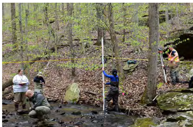
Measuring a reference reach with a team for a class project on Sharman's Branch in West Virginia.
