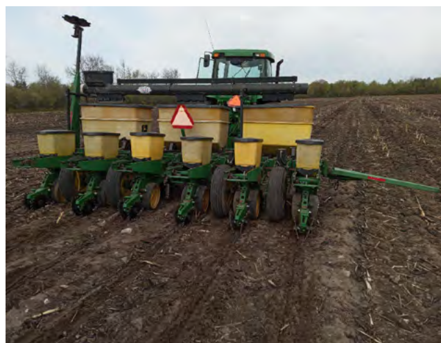
Planting corn without tillage with retrofitted planter
