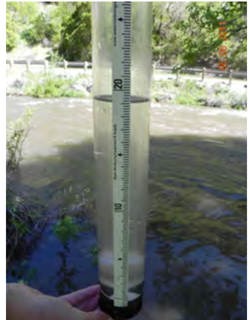
An example of a turbidity tube that MRBA will work with volunteers and/or students to construct.
