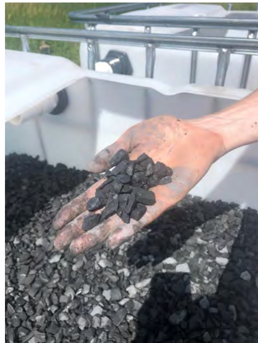
George Black media within the filter housing unit.
