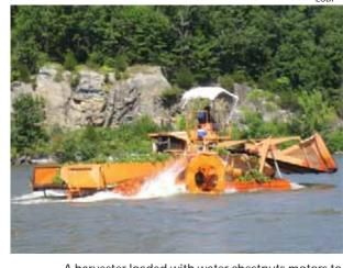
A harvester loaded with water chestnuts motors to a launch where the plants will be loaded onto dump trucks and hauled away for composting.
