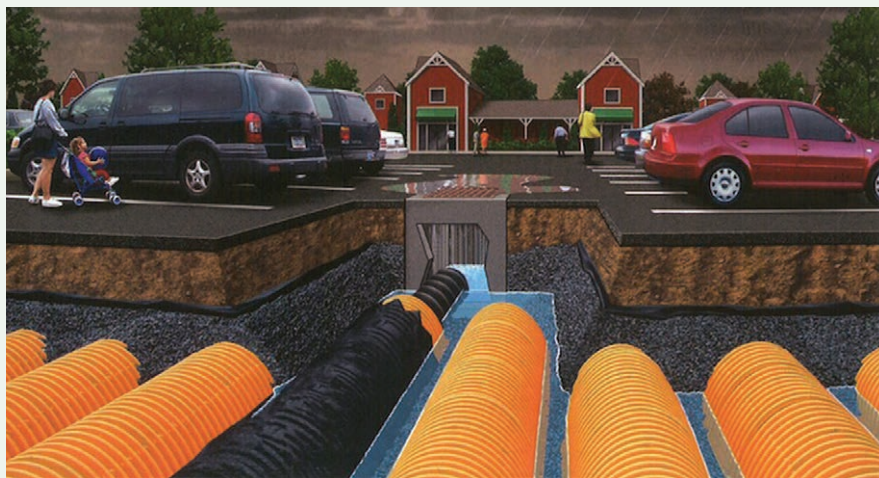
Image PE-14-1. This illustration shows sub-surface chambers installed below a parking lot.
