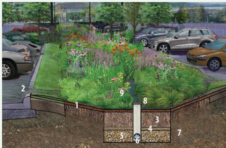
Image PE-11-1. The illustration shows a typical bioretention installed in a parking lot between parking aisles. This practice has an underdrain with a cleanout.
