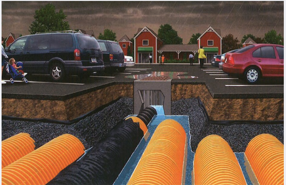
Image 4-CS-7-1. Concept illustration of underground storage chambers; sub-parking lot installations are common.
