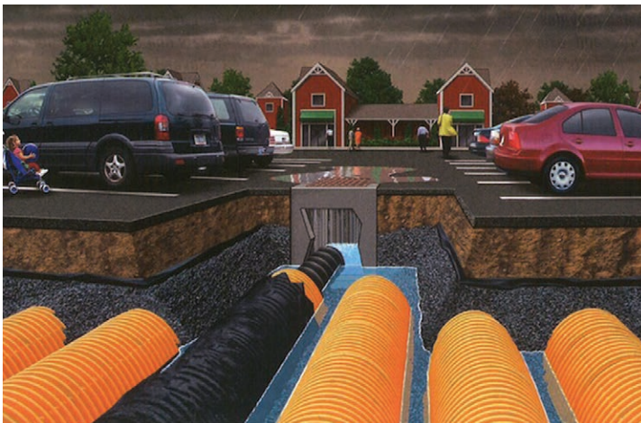
Image 1-4. Underground storage and infiltration chambers let site use continue without taking up space.
