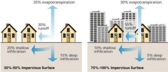
Fig. 3.21 — Relationship between impervious cover and surface runoff. Impervious cover in a watershed results in increased surface runoff. As little as 10 percent impervious cover in a watershed can result in
