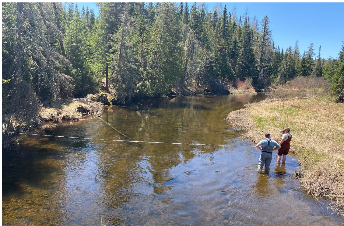
Figure 2. AWI Research Associate, Lija Treibergs, teaching an AWI Seasonal Research Technician and Paul Smith's College undergraduate student how to measure discharge using an acoustic Doppler velocimeter at the Lower Chubb River site.
