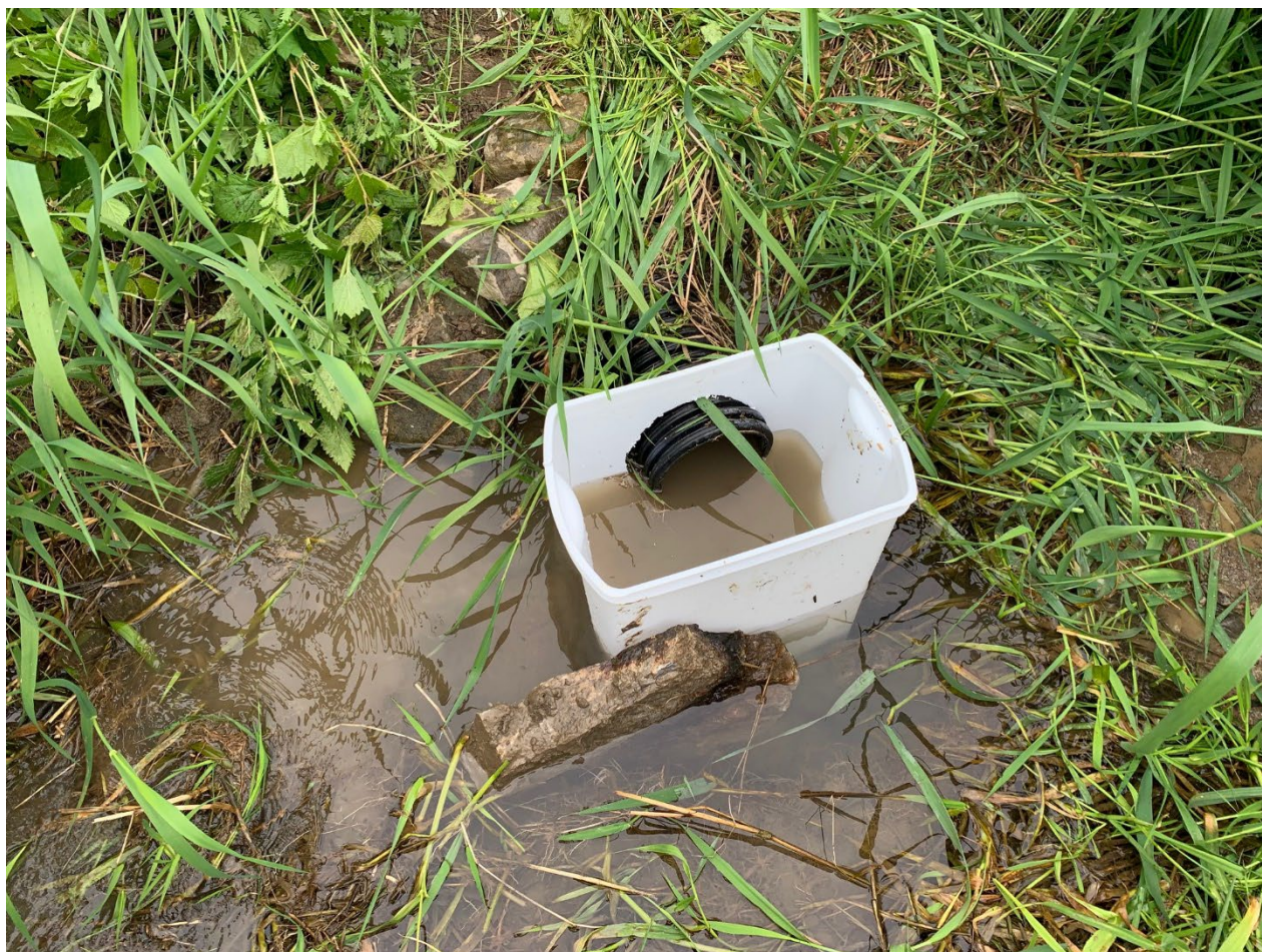
Figure 12. Close-up of sump collecting ditch flow.
