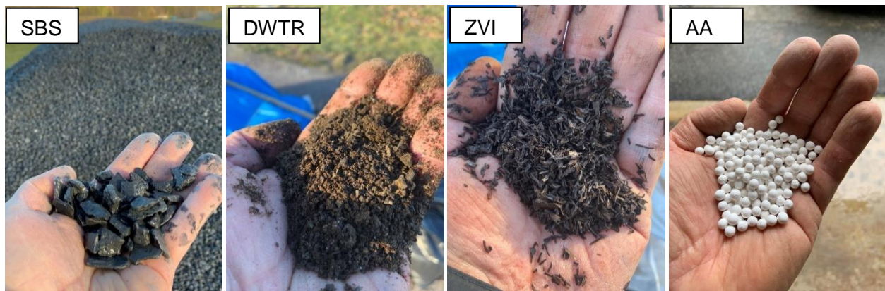
Figure 3. Filter media used in Dorset Park stormwater pond P filters
