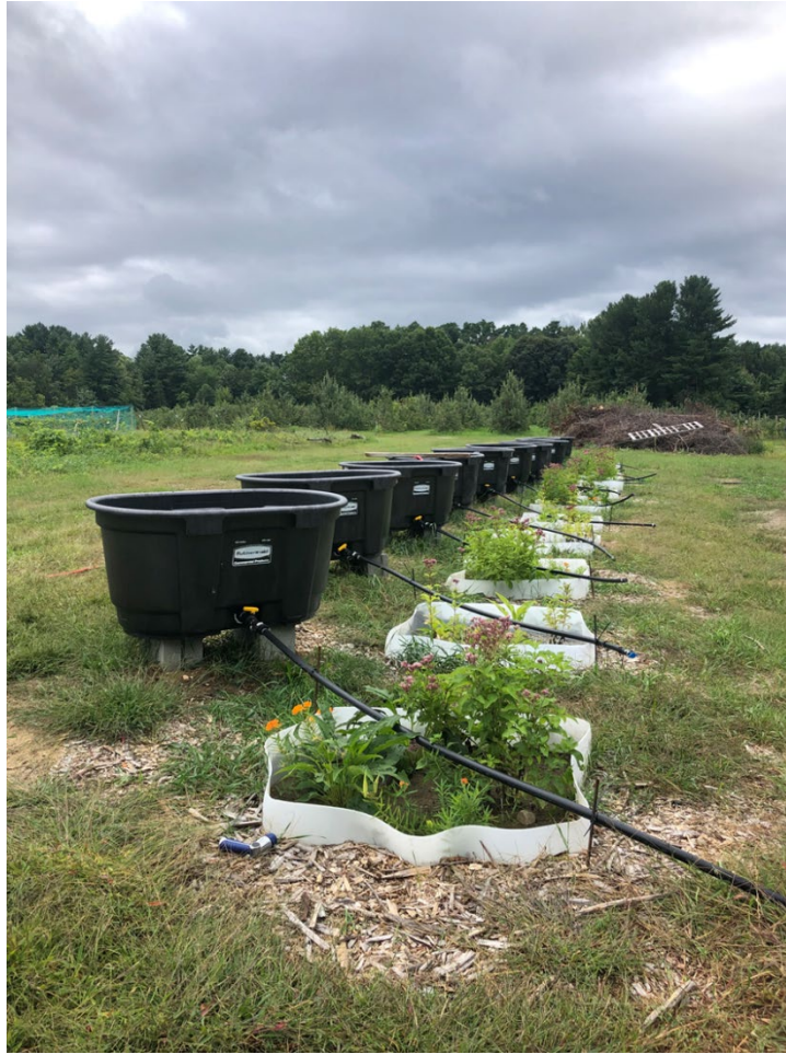
Figure 1. Photo of research site including twelve sets of influent tanks for mixing simulated stormwater, water distribution lines, and vegetated bioretention mesocosms. Photo by Samantha Brewer.
